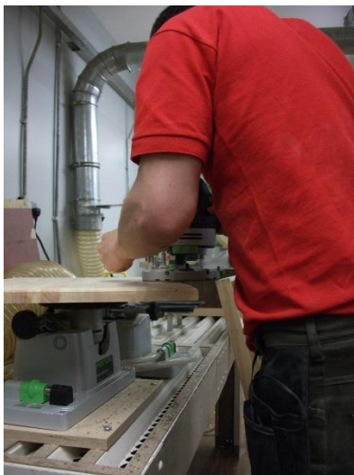
Event no. 30 – Using hand held router to mould edge on table top
