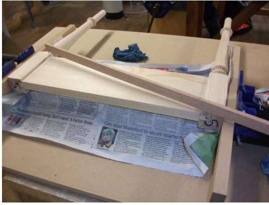
Event no. 25 and 26 – Gluing, clamping and checking for square
