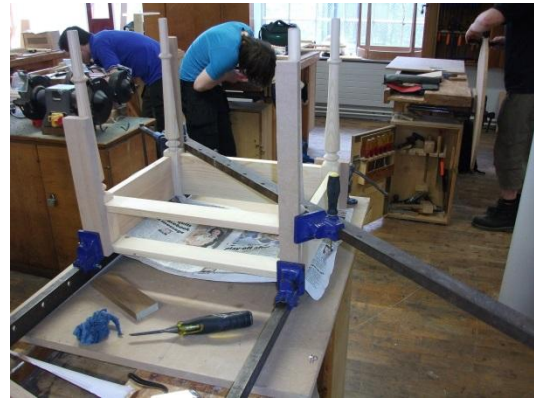
Event no. 25 and 26 – Gluing, clamping and checking for square
