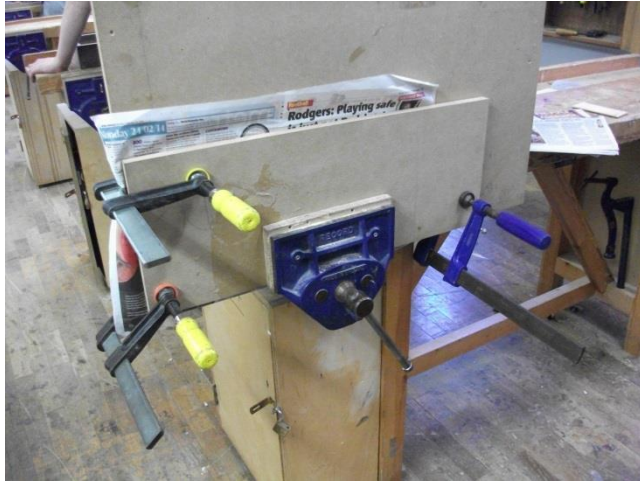
Event no. 29 – Balancing Veneer clamped in place while glue sets
