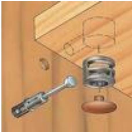
(Mini-fix) Bolt & Cam : Recessed & concealed, carcase and solid furniture
